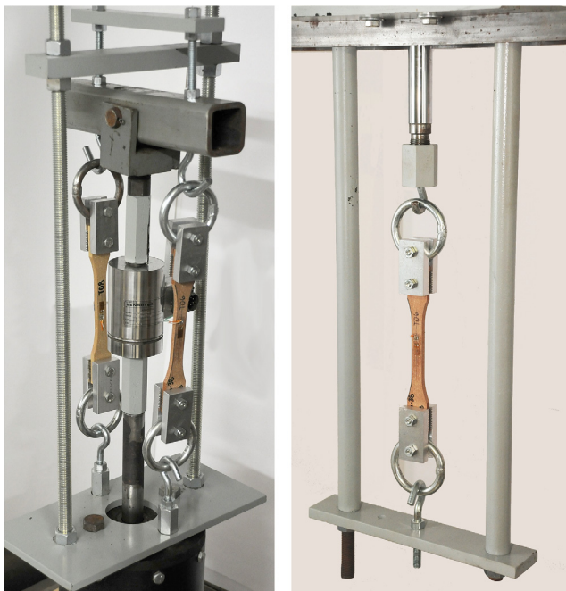
FIG. 2—Tension creep apparatuses: (a) single-specimen pneumatic loading and (b) two-specimen pneumatic loading.
