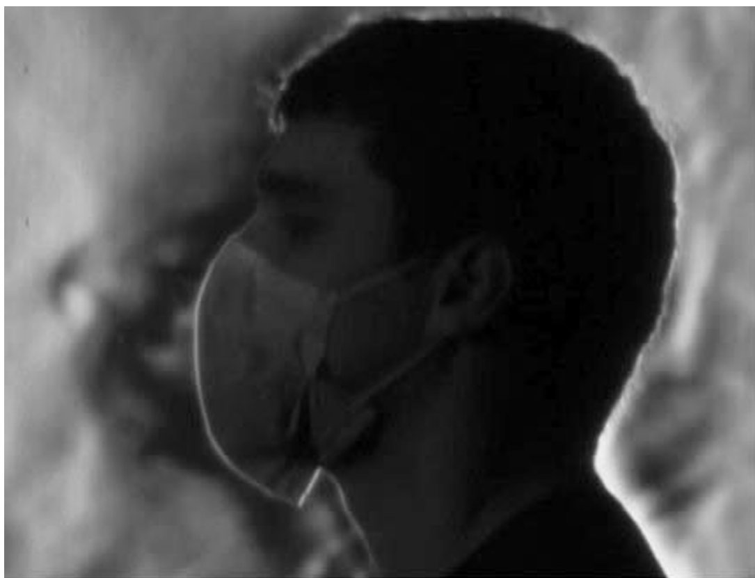
7 Schlieren optical imaging: Plumes of air from same individual as in Fig. 6 wearing PT mask. More air is exhaled through the mask with only a small amount of leak around the mask.
